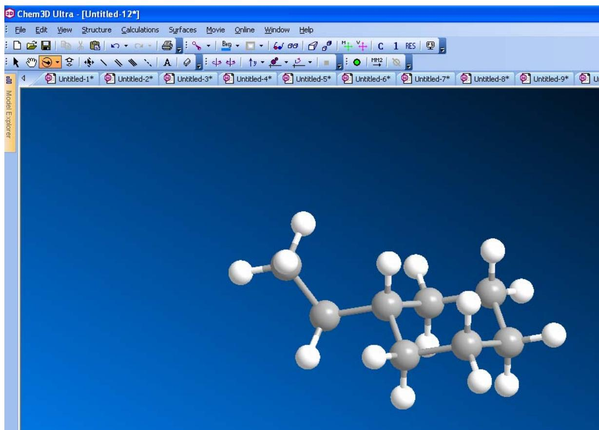
To change the position of the model on the screen you use the "hand" tool on the second row of the tool bar; the orientation of the model on the screen is altered by using the "rotate" tool, which is highlighted in orange on the above picture. Once you have the view and orientation you need you're ready to start doing energy calculations.
